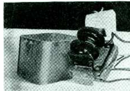
Attach a .1 mfd., 600-volt replacement in place of the old condenser, wrap it in paper to prevent warm tar from melting the insulation. Reheat the tar and restore the assembly to the "bath-tub," anchoring it with new rivets or small bolts
